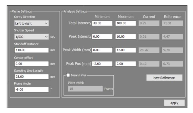
All the settings can be changed through the settings panel except for the "response time" which is located on the home screen above the acquisition and experiment control buttons.
