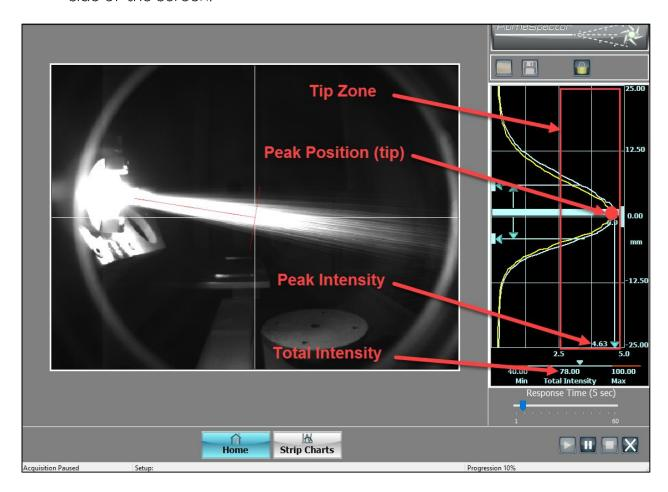
The camera measures intensity (arbitrary units). Those units are based on the shutter speed (exposure time) and the pixels saturation percentage. For example, if the shutter speed is 1 / 500s, the maximum intensity for 1 pixel is 5 A.U. We arbitrarily divided the denominator of the shutter speed by 100.
