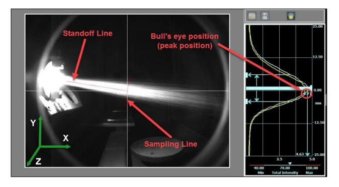
6. Adjust the "Plume Angle" so that the standoff line is perfectly centered on top of the plume. The standoff line should be parallel with the plume axis.
